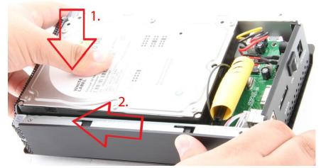
6. Place the cover back on the enclosure. Screw it back in place: Figure A:
